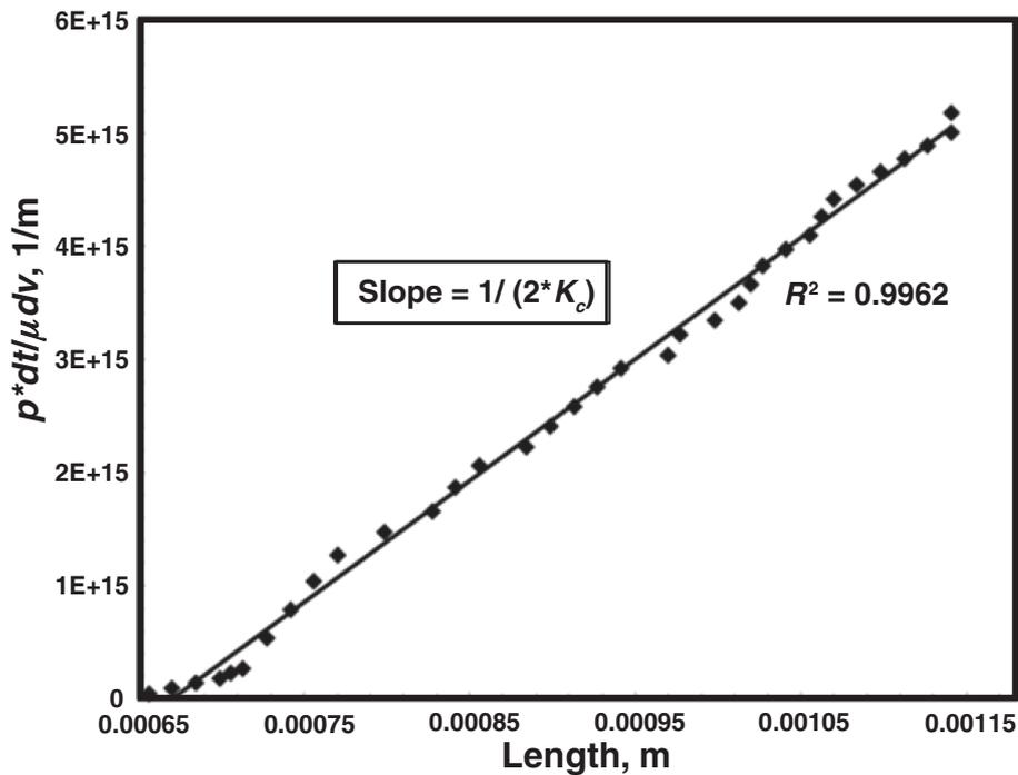
Fig. 14—Martinez et al. (2000) method used to determine the permeability of the filter cake.
