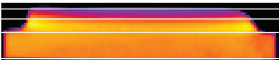
Fig. 6—Filter-cake layers of Drilling Fluid C with 10.3 ppg.
