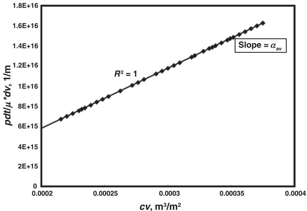
**Fig. 13—Tiller (2002) method used to determine the permeability of the filter cake.**
