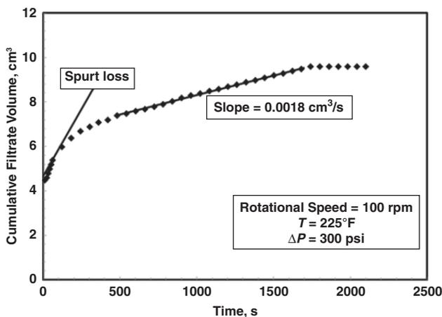
Fig. 17—Cumulative filtrate volume as a function of time of Drilling Fluid A under dynamic conditions (100 rpm).
