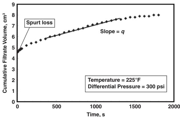
Fig. 15—Li et al. (2005) method used to determine the permeability of the filter cake.
