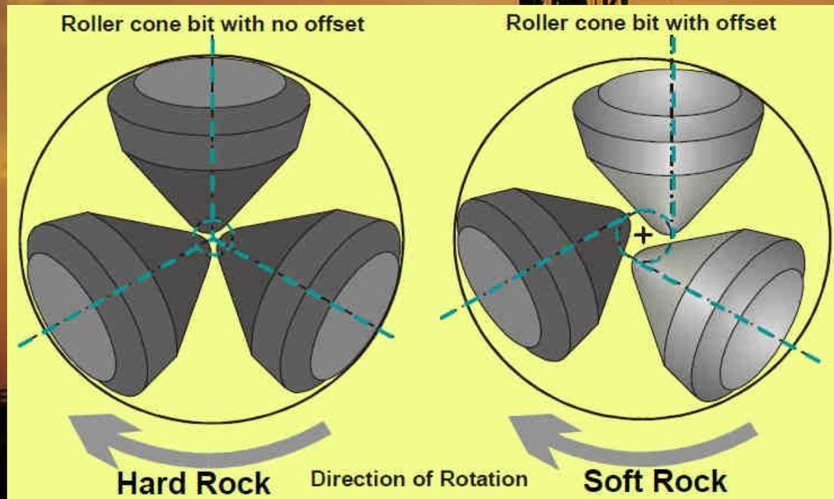
**Offset** of cones increases **Sliding, Tearing, Gouging** action
