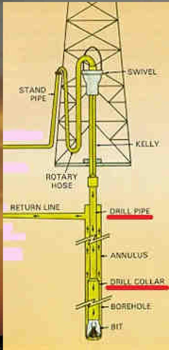
The **drill string** is the mechanical assemblage **connection** the rotary drive on **surface** to the drilling **bit on bottom** of the hole
