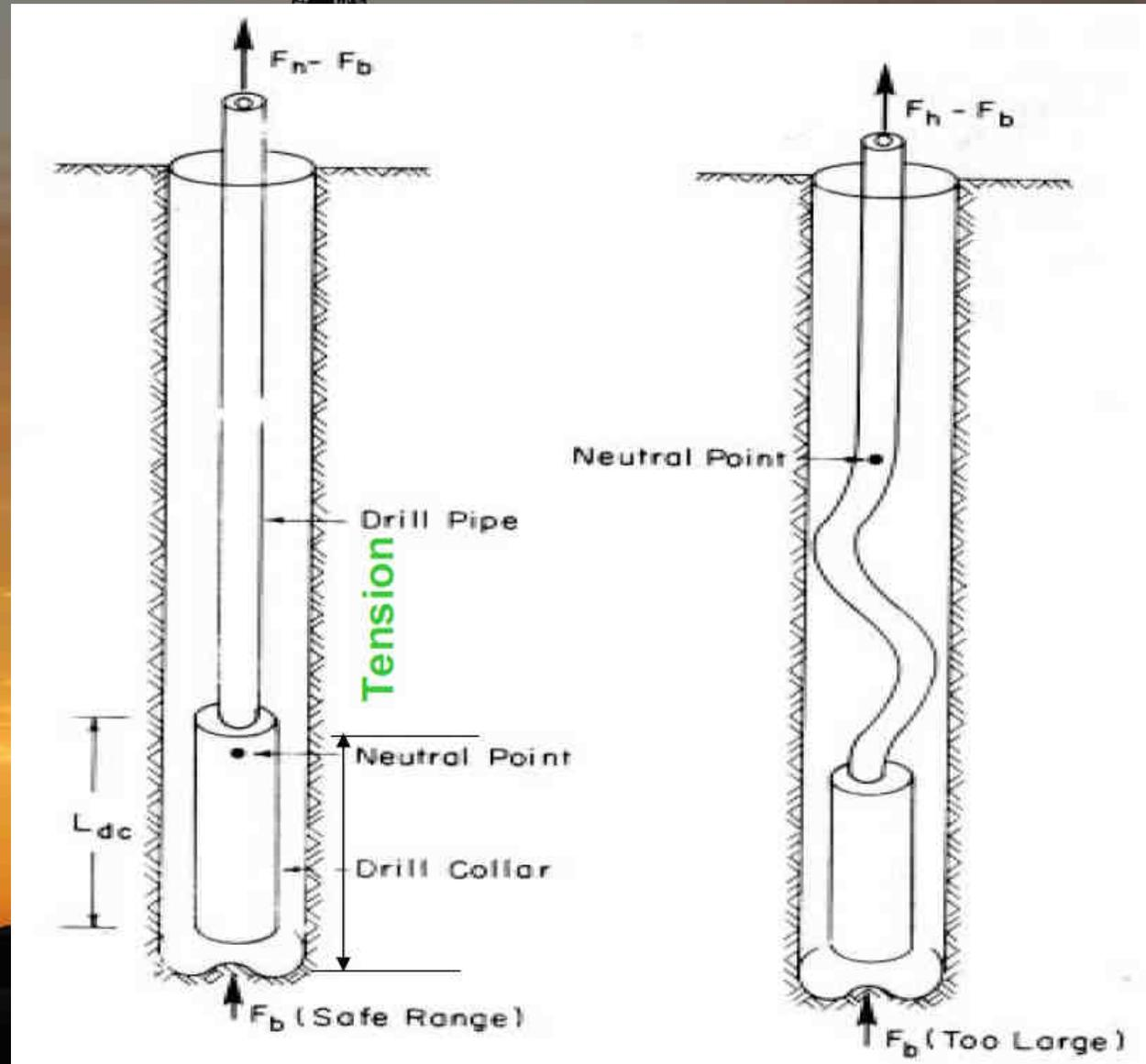
**Buckling of Drillpipe under Compressional Load!**
