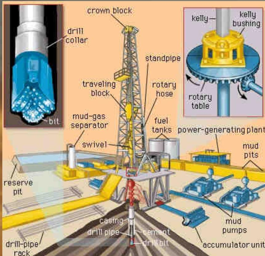
**Drilling Fluid** is circulated by being pumped down the **drill string**
