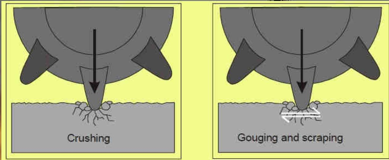
Cones of Roller Bits do only **roll** on the bottom but always **Slide, Tear and Gouge**
