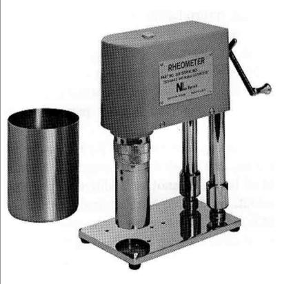
Determination of Shear Dependent Viscosity by Measuring Flow Curve at different Rotational Speeds Marsh Funnel
