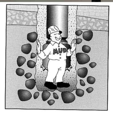
While Drilling Open Hole Mud Column should act as "Hydraulic Casing" Sufficient Mud Density
