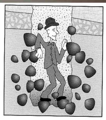
Insufficient Mud Density Bad Filtration Properties
